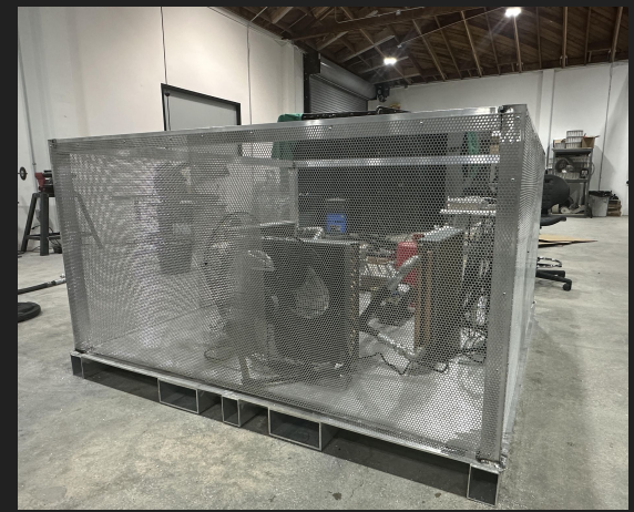
Full skid w/ perforated sheet enclosure
